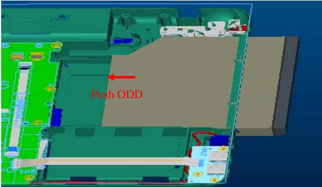
Figure 4-16-2 installing the Optical disc drive
