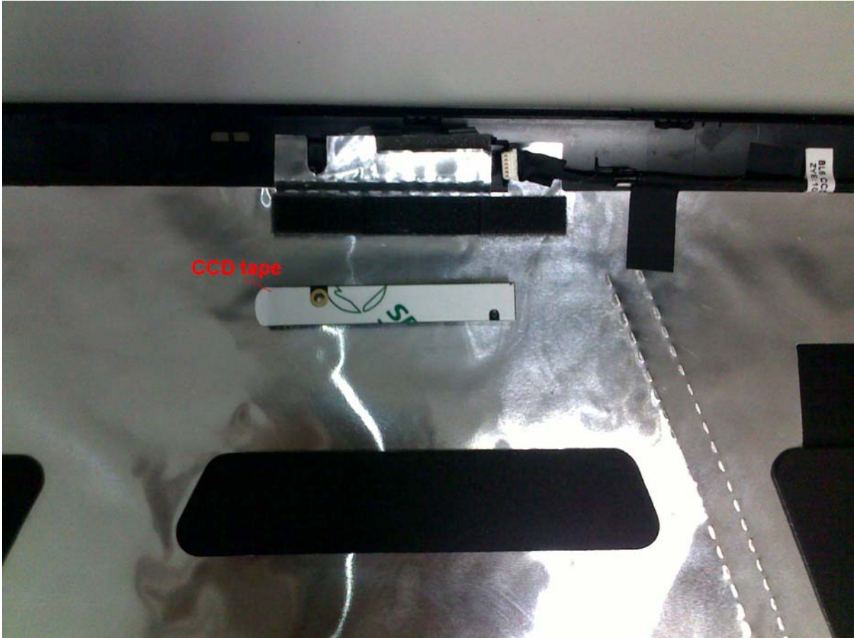
Figure 4-20-3 Camera Module before installing
